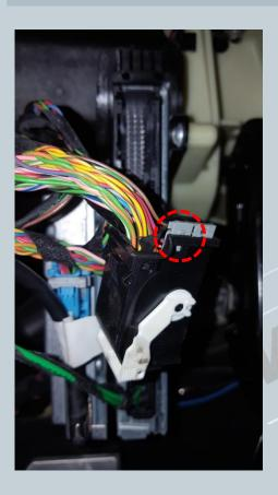
Unplug the black connector and pull it out of the connector housing. The housing is locked in place on both sides (marked in red).
