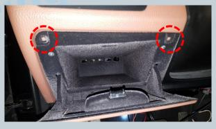
Loosen the 2 screws on the storage compartment and pull out the compartment.
