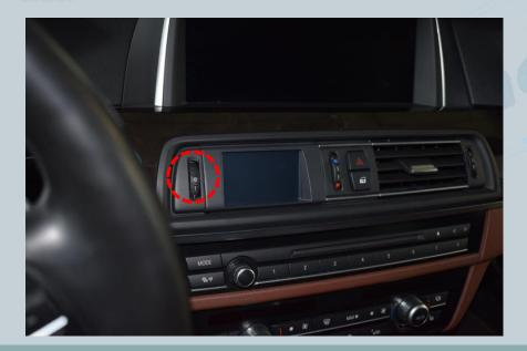
The interior trim strip can be clipped back into place. Start from left to right. Make sure it is in the correct position.
