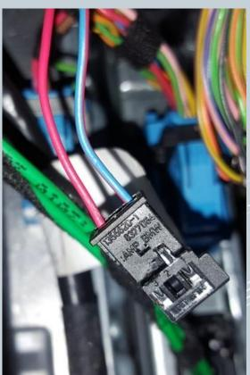
Plug the unpinned CAN cable into the connector supplied. Connect "blue/red" to **pin\_1** and "red" to **pin\_3**. The numbering is marked on the connector.
